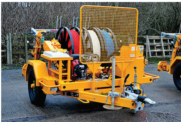
Puller for distribution lines
